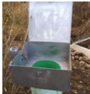
Stilling well cover / SDR equipment enclosure box
