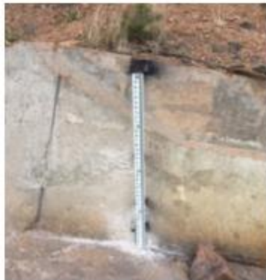
Installed staff gauge
